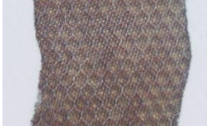
FIGURE 4: Coatings were removed from the P-3 Orion aircraft radome panel at a rate of 12 ft 2 /hr with no visual damage.
