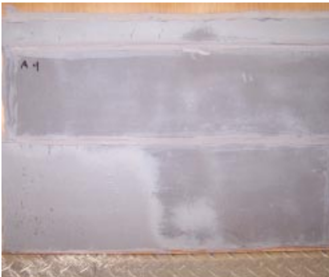
FIGURE 8: Coatings were removed from the PCMS radar-absorbing material at a rate of 35 ft 2 /hr with no visual damage.
