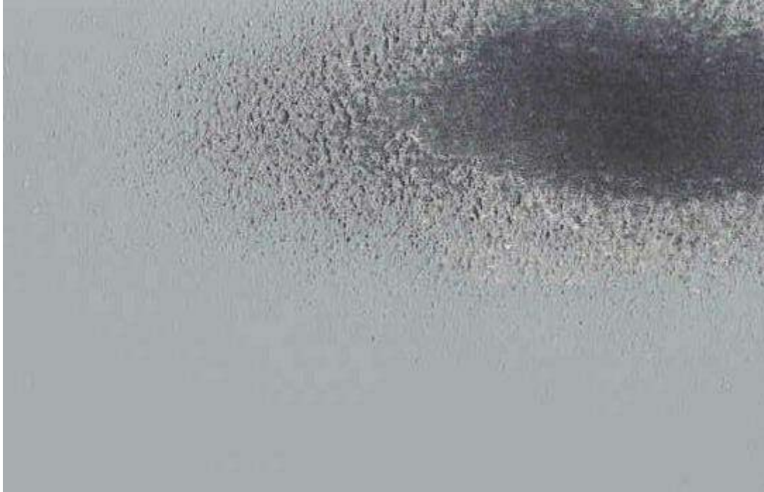
Photo 5: Fluoropolymer coating on carbon fibre substrate removed by GPX.
