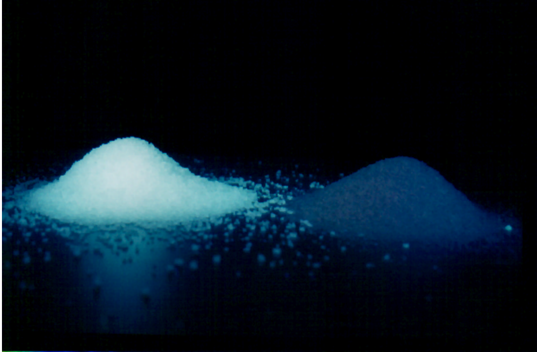
EXHIBIT 5, ultraviolet light response of XL series product (left) compared to type V plastic (right)
