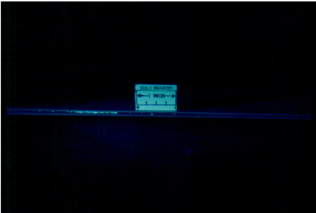
EXHIBIT 8, ultraviolet illumination of media ingress, XL on left-hand, type V on right-hand
