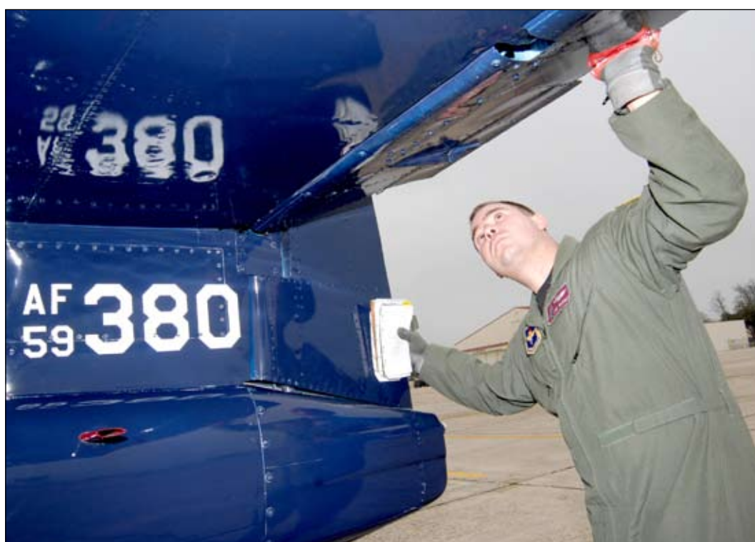
Capt. Joe Rucker, 559th Flying Training Squadron T-37 instructor pilot student, checks the aircraft's elevator during an exterior inspection check. (Photo by Melissa Peterson)
