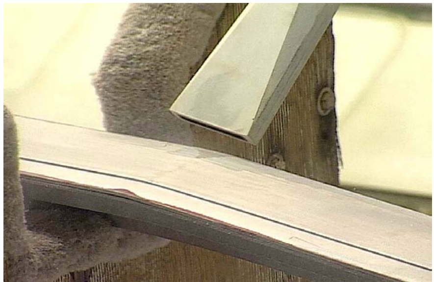
Flat Nozzle removing adhesive flash. (Photo courtesy of Pauli Systems)
