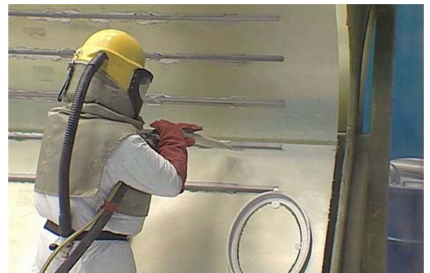
ABOVE: Operator applying the Envirostrip process to a large metal bonded structural part. (Photo courtesy of Pauli)
