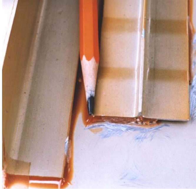
Damage caused by mechanical grinding.
